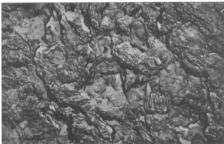
FIGURE 3 IMI 318 alloy etched with hydrochloric acid 10% at 103°C for 45 minutes. Original magnification \times 2500 .
