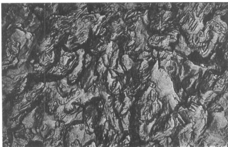
FIGURE 4 IMI 318 alloy etched with sulphuric acid 10% at 103°C for 45 minutes. Original magnification \times 2500 .
