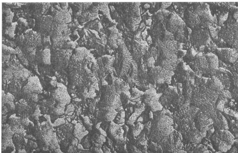
FIGURE 2 IMI 318 alloy etched with hydrofluoric acid 4% at 23°C for 1½ minutes. Original magnification \times 2500 .
